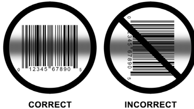
Figure 18. 1D Bar Code Orientation
