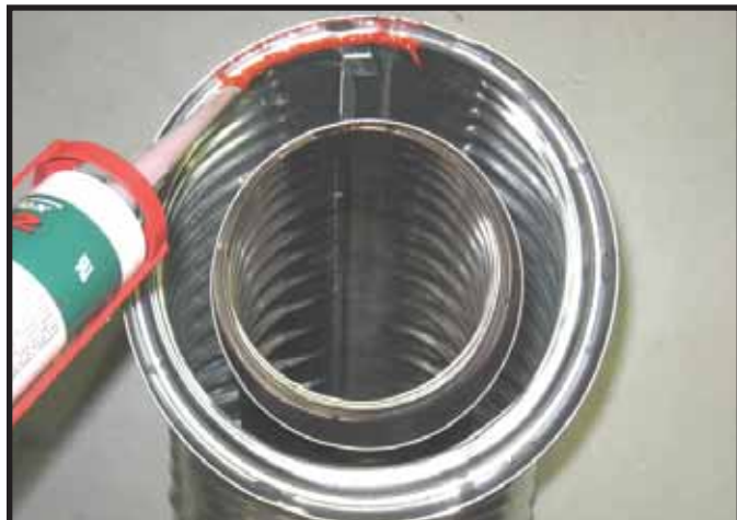
Figure 10.1 High Temperature Silicone Sealant
