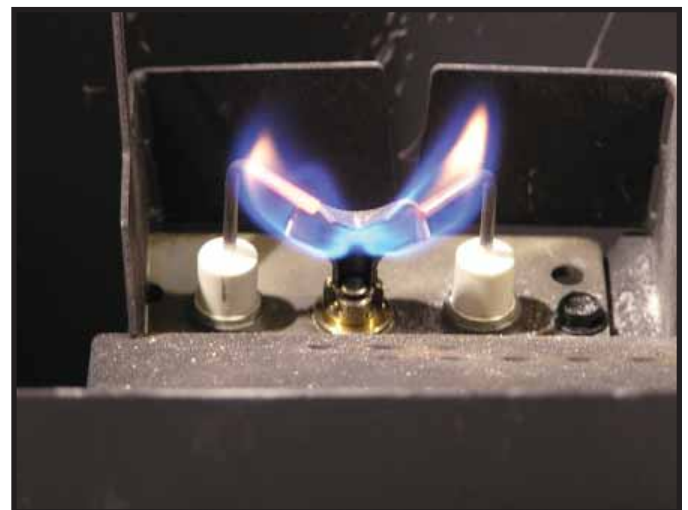
Figure 3.1 IPI Pilot Flame Patterns
