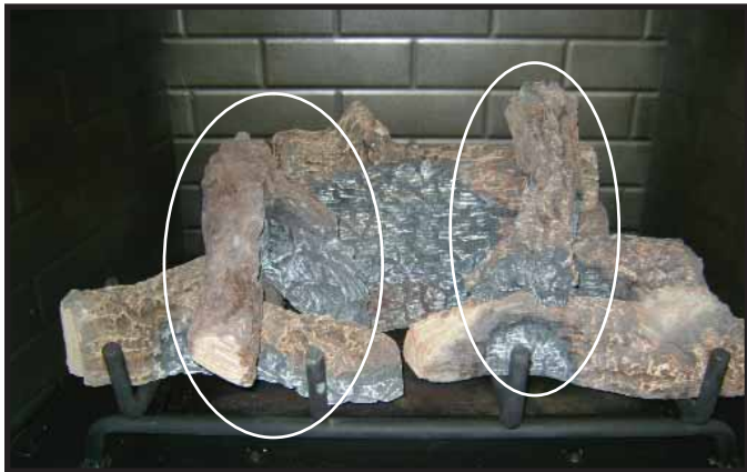
Figure 3.2 Remove Top Two Logs
