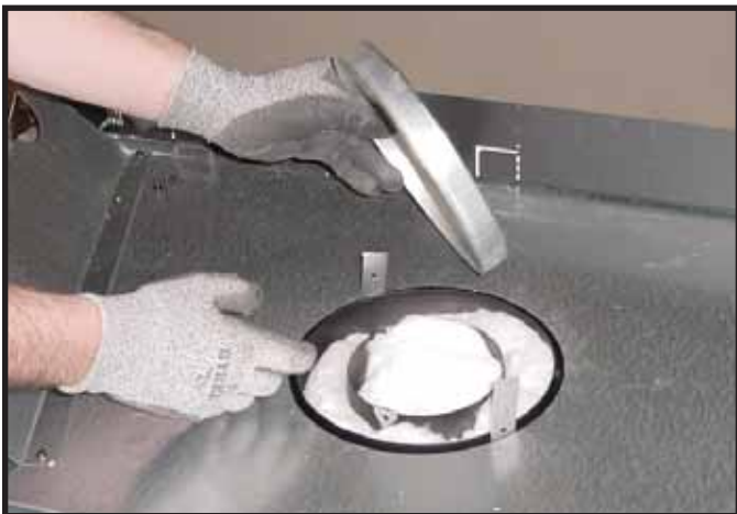
Figure 9.3 Remove the seal cap.
