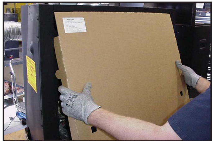
Figure 13.4 Installation of Splatter Guard
