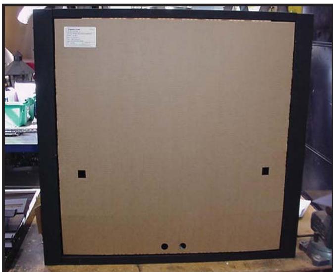
Figure 13.11 Splatter Guard with Lower Access Panel Closed
