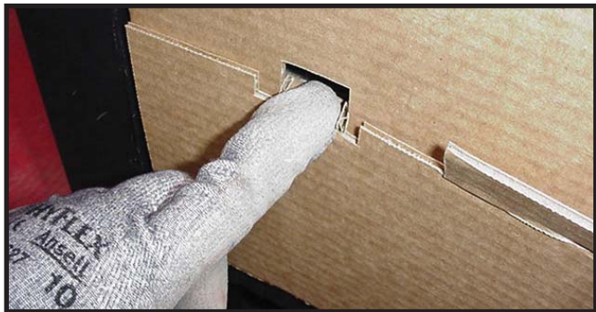
Figure 13.9 Securing Tabs Inside Front of Splatter Guard
