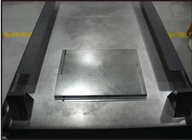
Figure 9.1 Remove the elbow heat shield by removing the four screws holding it to the top of the appliance. Refer to Section 6B to determine if the elbow heat shield is required.
