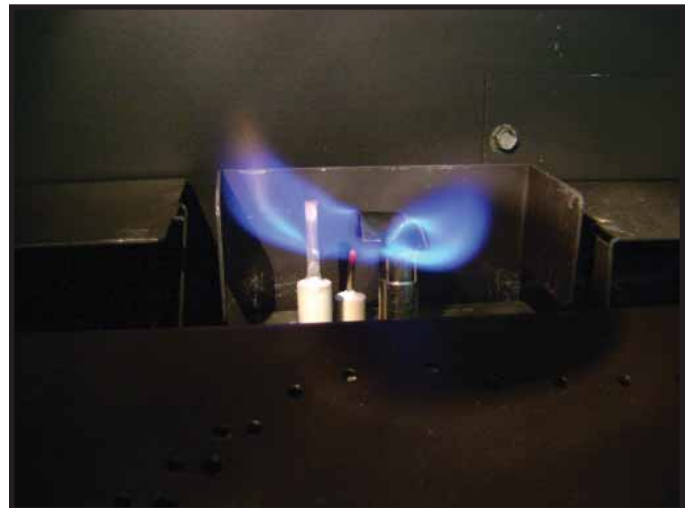
Figure 3.2 IPI Pilot Flame Patterns
