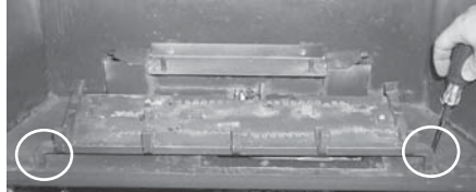
Remove the 2 screws, push Burner Assembly to the left and lift out.
