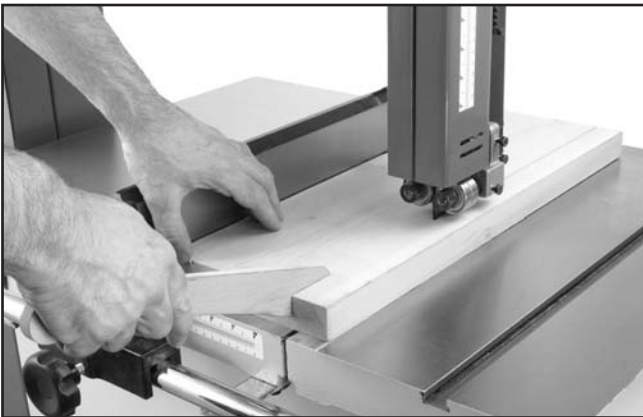
Figure 40. Example of typical ripping operation with a push stick.
