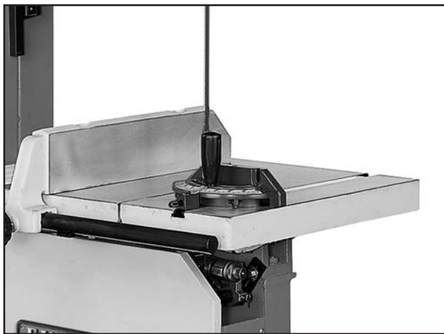
Figure 21. Miter gauge installed.
