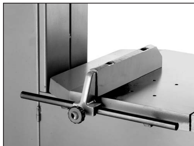
Figure 20. Fence mounted on rail.
