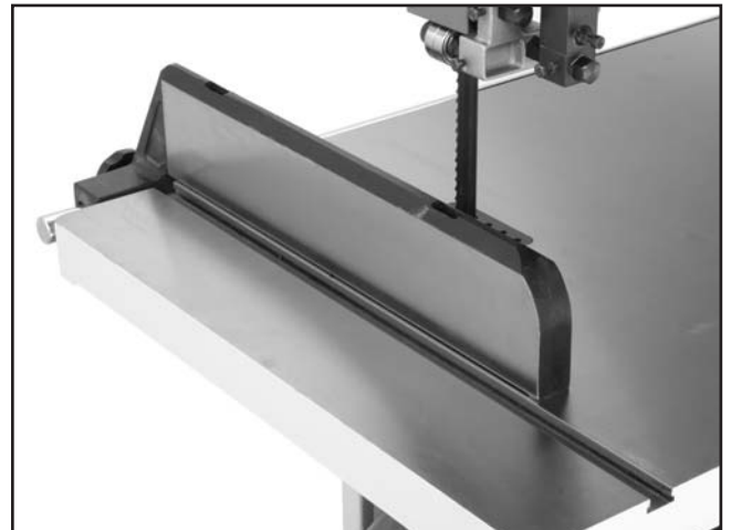
Figure 33. Typical example of fence parallel with miter slot.
