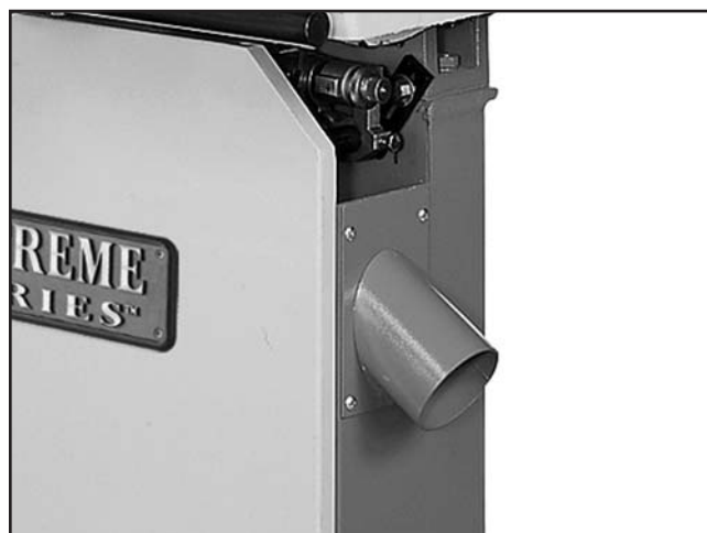
Figure 18. Dust port installed.
