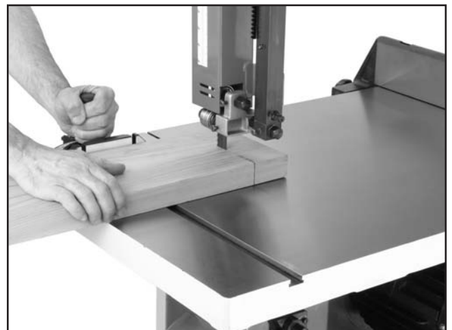
Figure 41. Example of crosscutting operation with miter gauge.
