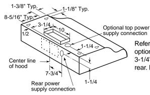
Refer to this drawing for rectangular exhaust option. Exhaust outlet connects to 3-1/4" x 10" rectangular duct. Vent top or rear. Includes rectangular damper.
