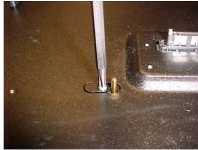
Single Cap positioned to block WLAN contact
