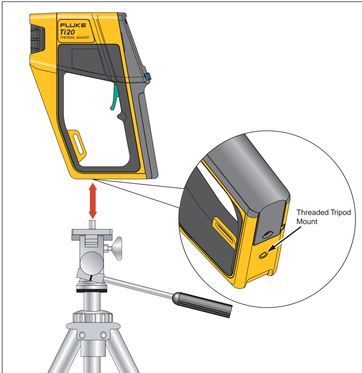
Figure 1-10. Mounting the Imager on a Tripod
