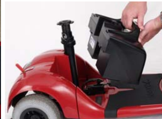
Remove battery box.
