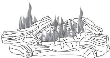
Figure 39 - Incorrect Flame Pattern with Control Knob Set to High Flame
