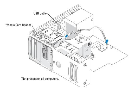
5 Disconnect the USB cable on the back of the Media Card Reader to the front panel USB connector on the system board (see page 71) and route the cable through the clip on the shroud.
