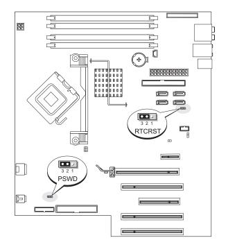
2 Locate the 3-pin password jumper (PSWD) on the system board (see page 71), and attach the jumper plug to pins 2 and 3 to clear the password.
