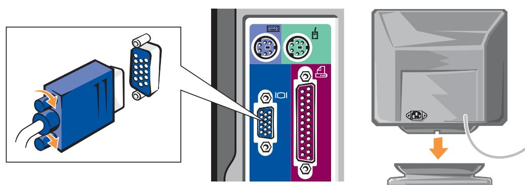
Align and gently insert the monitor cable connector. Do not bend the connector pins. Then tighten the thumbscrews.
