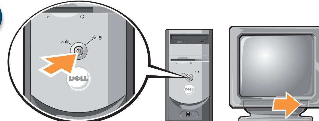
Press the power buttons to turn on your computer and monitor. Then turn on the speakers and/or subwoofer (if necessary). Follow the instructions on the screen to complete the Microsoft Windows operating system setup.
