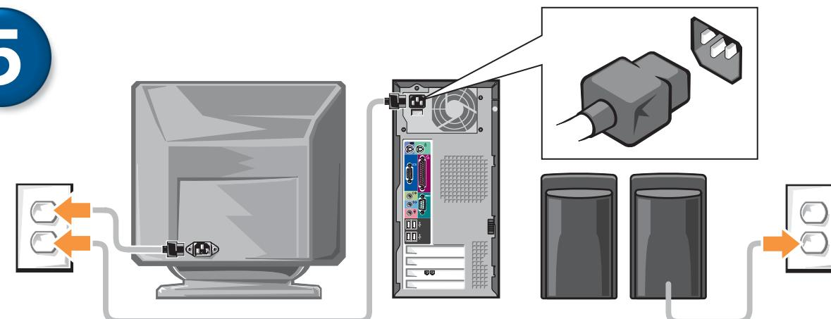
Connect the monitor, computer, and speaker system to electrical outlets.
