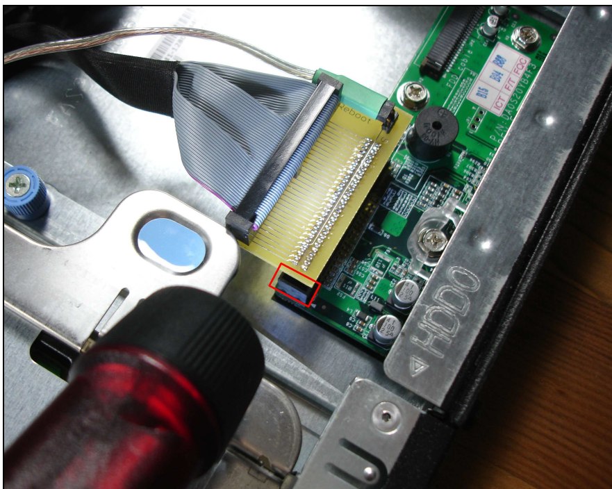
Figure 16 - Ensuring that the Adapter Board is Properly Aligned with the Front Panel Board
