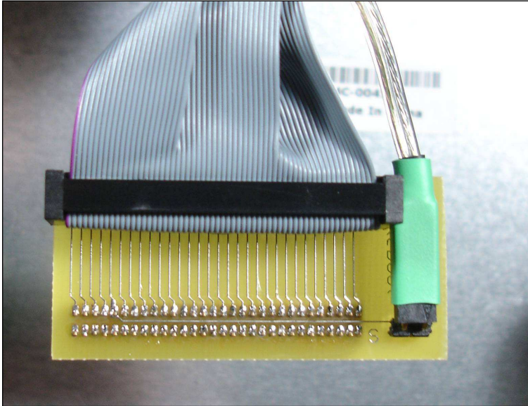
Figure 14 – Connecting the Motherboard Cable to the Adapter Board
