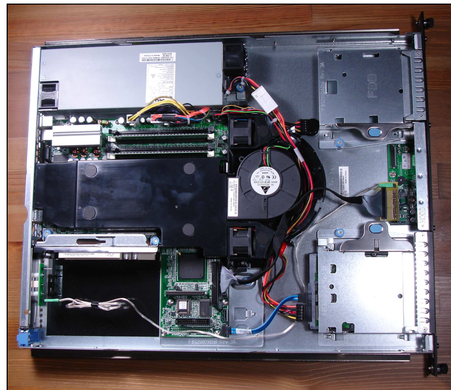
Figure 17 – Completed Adapter Board Installation
