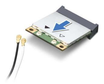
CAUTION: When the Mini-Card is not in the computer, store it in protective antistatic packaging. For more information, see "Protecting Against Electrostatic Discharge" in the safety information that shipped with your computer.
