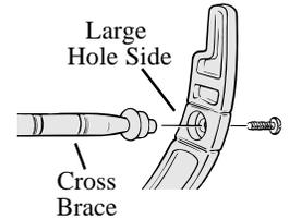
**CAUTION:** Inserting cross braces in wrong side of leg (small hole side) can cause cross braces to break during use.
