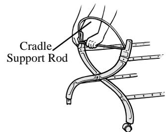
Make sure rod installed in steps 3 & 4 remains hooked on cross braces before securing cradle supports.
