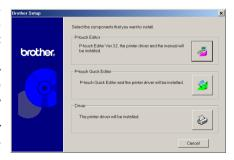
3 Click the lower button (Driver). A Driver Setup dialog box appears, allowing you to select whether to replace, add or delete the PT-2600/2610 printer driver.
