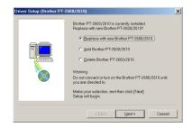
If "Replace with new Brother PT-2600/2610" is selected, the previously installed printer driver is deleted, and replaced with a new one. Select this option when upgrading the printer driver, or when running Windows 2000 or XP and changing to a P-touch 2600/2610 with a different serial number.
