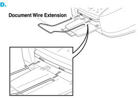
A. Fan the paper well. Gently insert the paper. Make sure the print side is toward you and the paper level is stacked below the paper guide line. Paper Guide Line B. Press and slide the guide to fit the paper width **Paper Width Guide**
