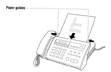
■ The automatic document feeder (ADF) can hold up to 10 pages, feeding each one individually through the fax machine. Use standard (20 lb.) paper when using the ADF, if you're using heavier paper, feed each sheet individually to prevent paper jams.
