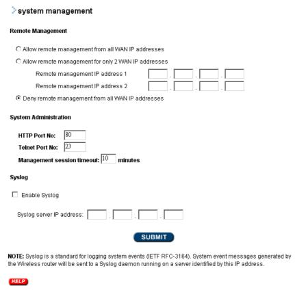
**Remote Management:** In this section, you can place restrictions on remote devices allowed to manage the router. You have three choices:
