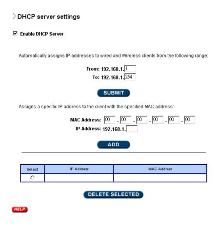
**Enable DHCP server:** To enable the DHCP server and allow the router to automatically assign private IP addresses to requesting device, check this box.
