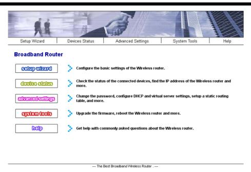
The home page displays the main menu on the upper-side of the screen; the main menu links are used to navigate to other menus that display configuration parameters and status. The Router management system includes Setup Wizard, Device Status, System Tools, Advanced Settings and Help choices.
