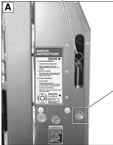
Manual Backup Pump
