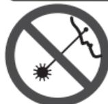
Do not direct the laser beam at persons or animals and do not stare into the laser beam yourself. This tool produces laser class 2 laser radiation and complies with 21 CFR 1040.10 and 1040.11 except for deviations pursuant to Laser Notice No. 50, dated June 24, 2007. This can lead to persons being blinded.
