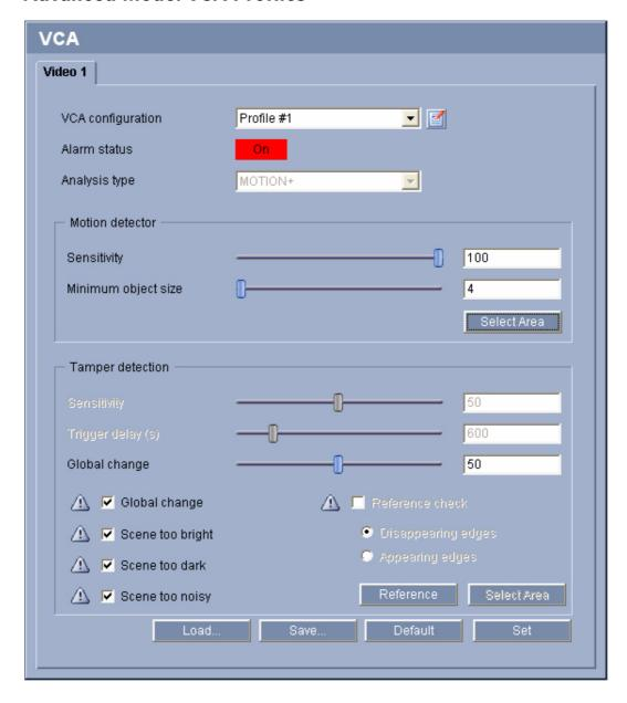
You can configure two profiles with different VCA configurations. You can save profiles on your computer's hard drive and load saved profiles from there. This can be useful if you want to test a number of different configurations. Save a functioning configuration and test new settings. You can use the saved configuration to restore the original settings at any time.
