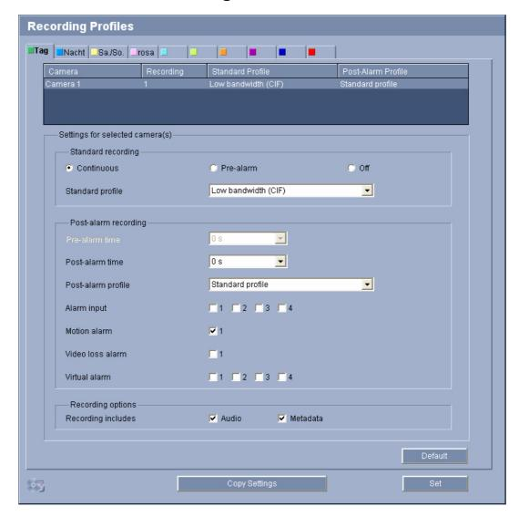
You can define up to ten different recording profiles. You will then use these recording profiles in the recording scheduler, where they are linked with the individual days and times (see Section 5.25 Advanced Mode: Recording Scheduler, page 56).
