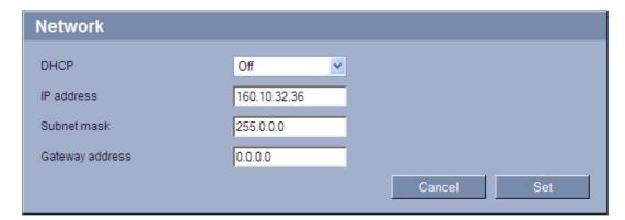
The settings on this page are used to integrate the VideoJet X10 SN into an existing network. Some changes only take effect after the unit is rebooted. In this case, the **Set** button changes to **Set and Reboot**.
