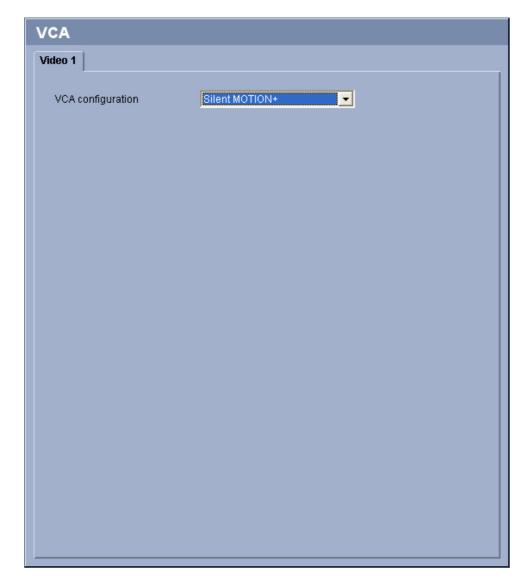
The VideoJet X10 SN contains an integrated video content analysis (VCA), which can detect and analyze changes in the signal on the basis of image processing. Such changes can be due to movements in the camera's field of view.
