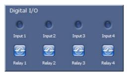
The alarm icons **Input 1** to **Input 4** are for information purposes and indicate the status of an alarm input: When an alarm is triggered, the corresponding icon lights up blue. The unit's configuration determines whether the alarm is displayed, as well as additional details (see *Section 5.15 Advanced Mode: LIVEPAGE Functions, page 42*).
