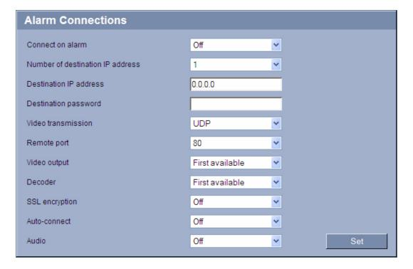
You can select how the VideoJet X10 SN responds to an alarm. In the event of an alarm, the unit can automatically connect to a pre-defined IP address. You can enter up to ten IP addresses to which the VideoJet X10 SN will connect in sequence in the event of an alarm, until a connection is made.
