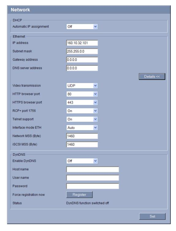
The settings on this page are used to integrate the VideoJet X10 SN into an existing network. Some changes only take effect after the unit is rebooted. In this case, the **Set** button changes to **Set and Reboot**.
