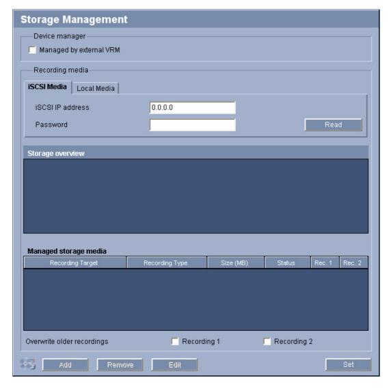
You can record the images from the camera connected to the VideoJet X10 SN on various local storage media or on an appropriately configured iSCSI system.
