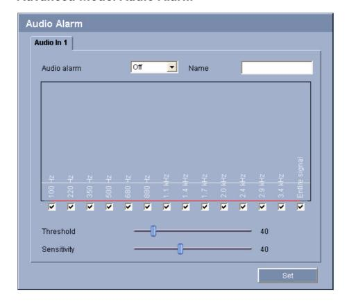
The VideoJet X10 SN can create alarms on the basis of audio signals. You can configure signal strengths and frequency ranges in such a way that false alarms, for example due to machine noise or background noise, are avoided.
