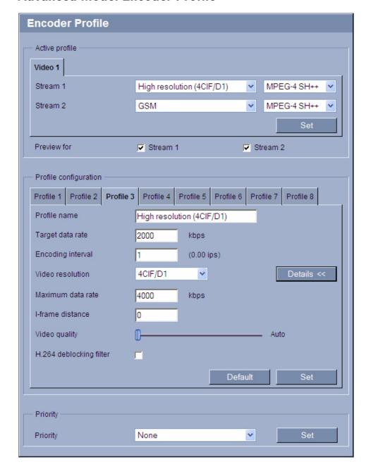
For the video signal encoding, you can select a code algorithm for each and two profiles, and you can change the presets for the profiles.
