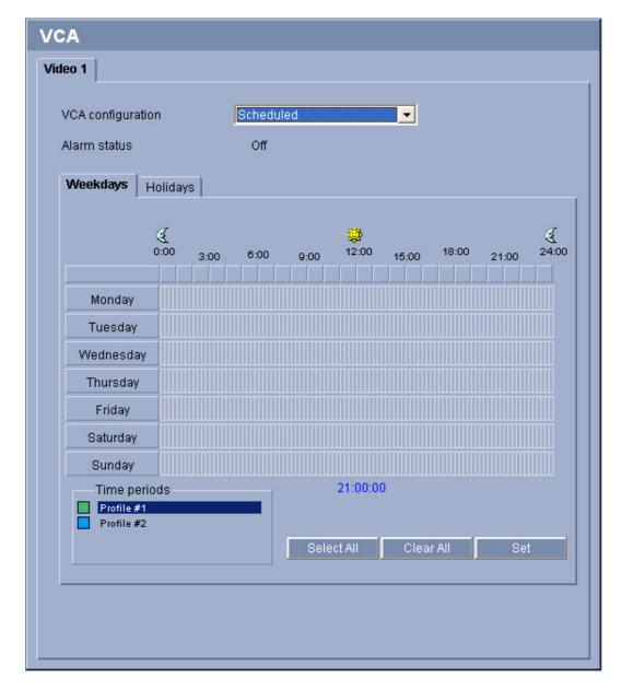
This configuration allows you to link the created VCA profile with the days and times at which the video content analysis is to be active.
