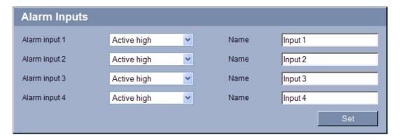
You can configure the alarm inputs of the VideoJet X10 SN.
