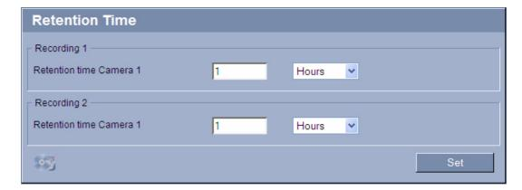
You can specify the retention times for recordings. If the available memory capacity of a medium has been used, older recordings are only overwritten if the retention time entered here has expired.
