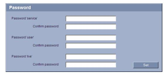
A VideoJet X10 SN is generally protected by a password to prevent unauthorized access to the unit. You can use different authorization levels to limit access.
