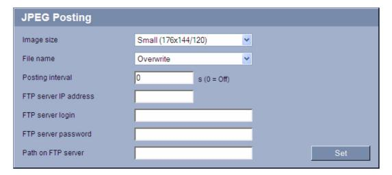
You can save individual JPEG images on an FTP server at specific intervals. You can then retrieve these images at a later date to reconstruct alarm events if required.
