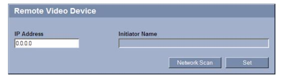
You can allow a remote video device to use the VideoJet X10 SN storage media. This means you can record video images from a camera that does not have its own storage media, for example. Once you have entered the IP address of the remote video device and saved it by pressing **Set**, the VideoJet X10 SN is then displayed for selection in the Storage Management for the remote video device.
