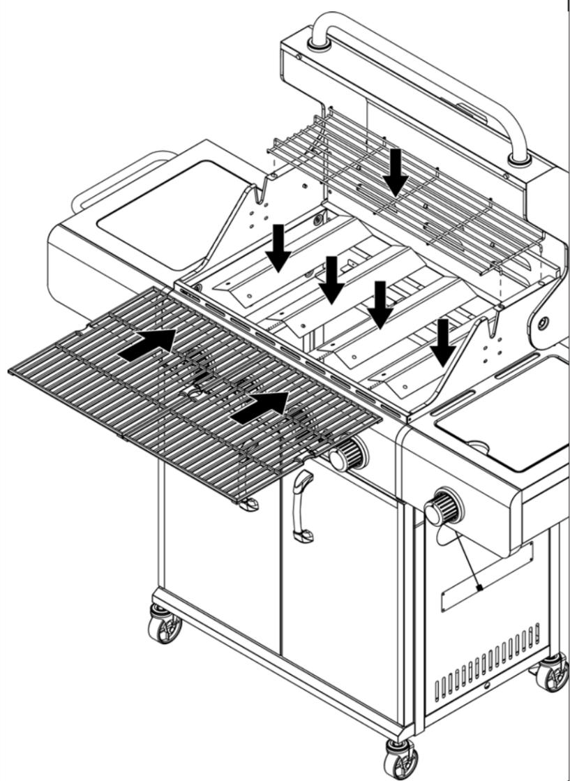
19 Insert Grease Tray Cup and Grease Tray
