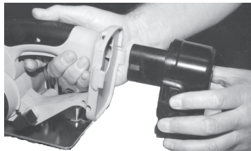
Figure 1-Installing the Battery Pack Assembly
