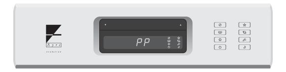
The chosen input is now programmed for "Processor Pass-Through" operation, disabling the now redundant volume control of the AX-7e. When that input is selected, the preamplifier section of the AX-7e is set to unity gain (0 dB), and the volume is controlled directly from the surround-sound processor. The volume indicator of the AX-7e will display "PP" to show that the "Processor Pass-Through" mode has been selected for that input.
