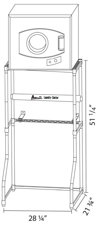
Your Washer / Dryer Stacking Bracket is designed to accommodate both top loading or front loading washing machines. Follow the assembly instructions below to assemble the bracket to fit your specific washing machine type. Images shown in this instruction guide are for assembly for use with a TOP-Load washer.
