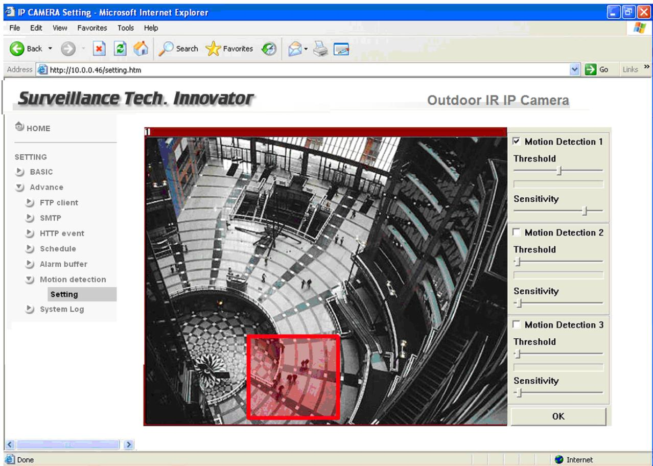
Click it **On** when you use the Motion Detection function and detecting zone appears for adjusting and moving. The common setting options are displayed below. If you do not wish to use the Motion Detection function, click it **Off** and press **OK**.
