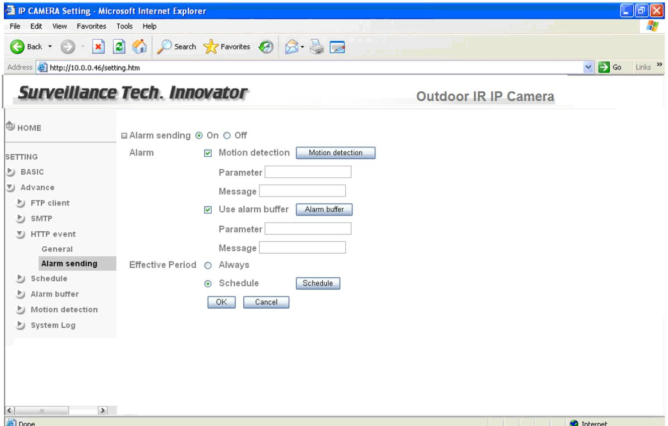
**Alarm sending** : Select **On** to set to send mail with connection to the alarm detection.
