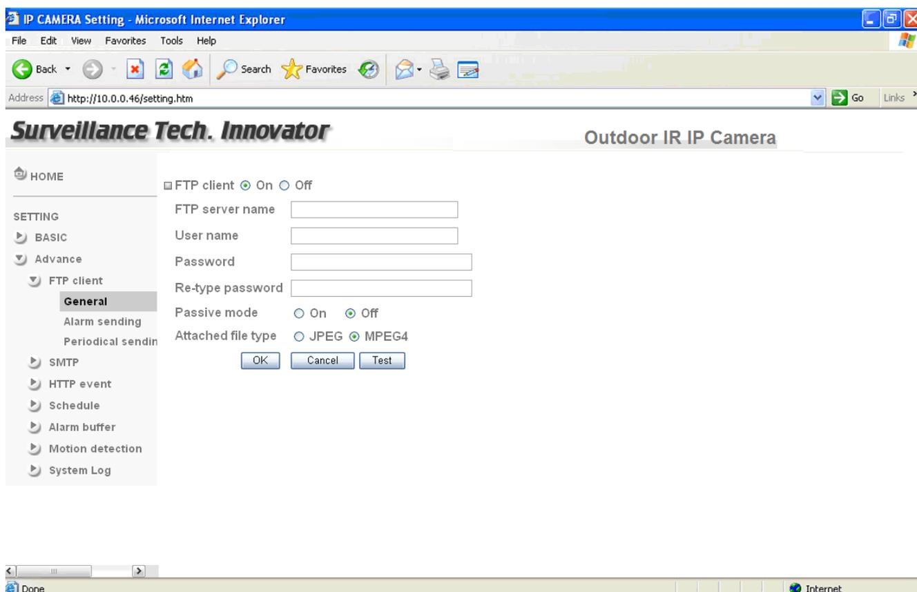
**FTP client function** : To activate the FTP client function, select **On**. The FTP client setting page appears. When you do not wish to use the FTP client function, select **Off**.
