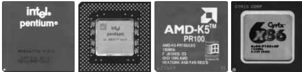
Intel P54C Pentium (75-200MHz) Intel P55C Pentium MMX (200MHz) AMD-K5 (PR75-133MHz) Cyrix 6x86 166+ Rev2.7 (133MHz)
