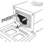
book, will now need to be fitted. Hook the bottom of the plate «A», into position first. Then push the other end of the plate into position.
