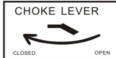
Figure 5 - Choke Lever in the "closed" position. (Refer to the Generator Components chart to find the location of the Choke Lever.)
