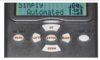
**BUTTONS:** The buttons provide easy navigation through the Pocket Programmer's menus on the LCD display.
