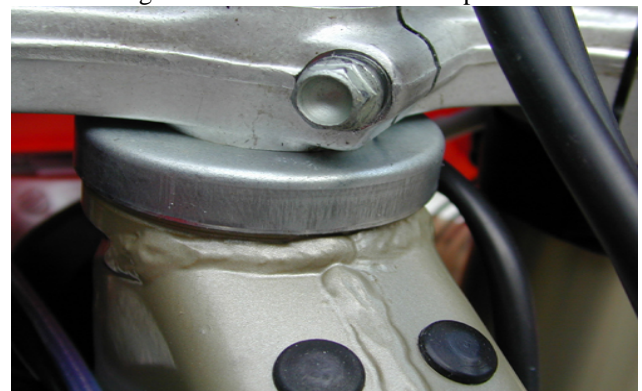
This sample would need a lot of filing at the weld
