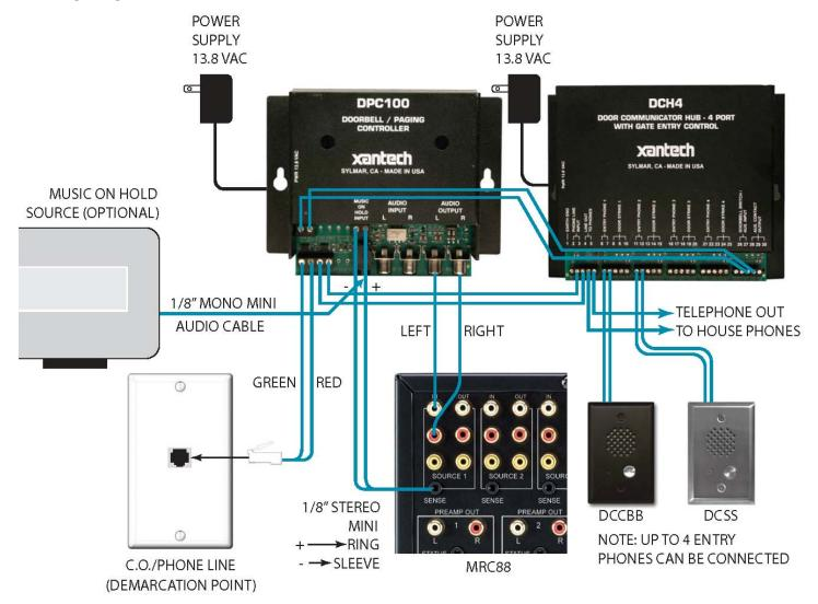
Note: DIP switch 2 must be 'on' (DPC100), DIP switch 1 must be 'off' (DCH4)
