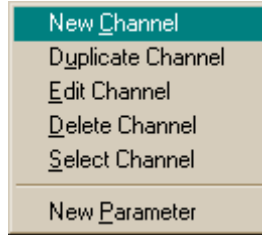
Figure 4-2: iDAS Channel Context Menu – Adding or Modifying a Channel
