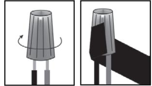
**5A. FOR SINGLE POLE APPLICATION ONLY:** Connect the **BLUE** wire of the HA14WD to the **LOAD** wire using a twist connector (provided.)
