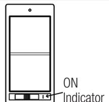
**NOTE:** When changing a light bulb, slide the air-gap switch to the **OFF** position. The **OFF** position is indicated if there is an "O" (**OFF** symbol) visible to the left of the air-gap switch. This disconnects electrical power to the light fixture to prevent an electrical shock. When the bulb has been replaced, slide the switch back to the **ON** position.
