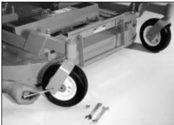
Deck Caster Wheel Installation
