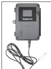
Cable from "AV Out"
