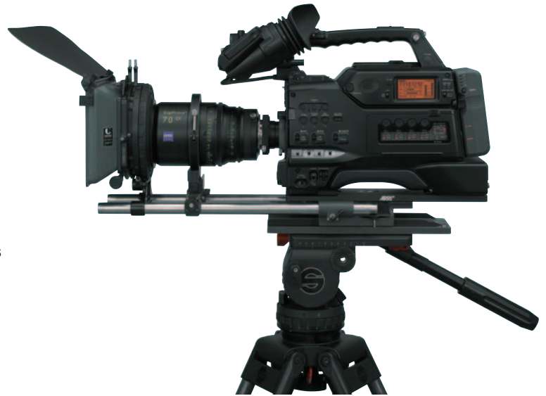
Cinema lens on HVR-S270U with an adaptor
