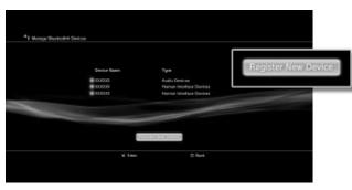
Scroll down and press **X** on the icon labeled *Manage Bluetooth Devices*. Select **Yes** to register a new device (if this is the first time registering a Bluetooth device) then press **X** on *Start Scanning*.
