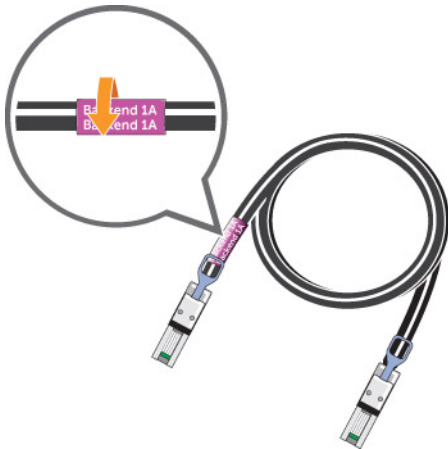
Figure 62. Wrap Label Around Cable
