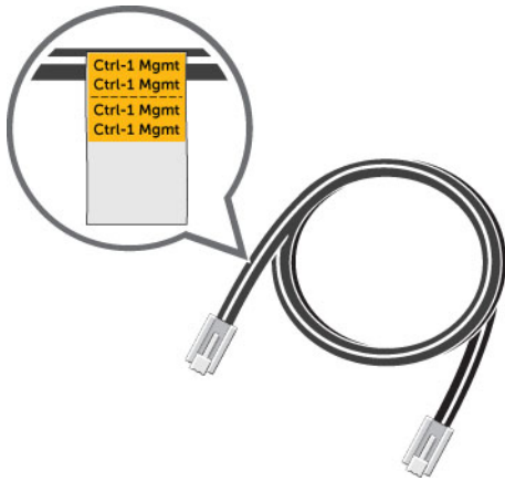
Figure 51. Attach Label to Cable
