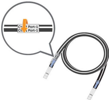
Figure 49. Wrap Label Around Cable
