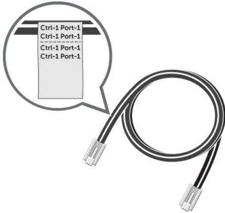
Figure 43. Attach Label to Cable
