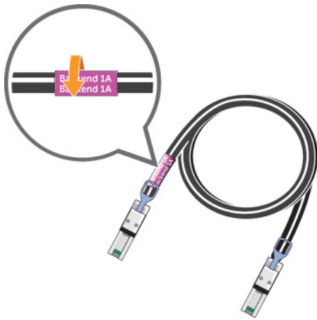
Figure 72. Wrap Label Around Cable
