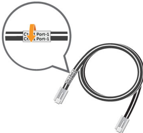
Figure 44. Wrap Label Around Cable
