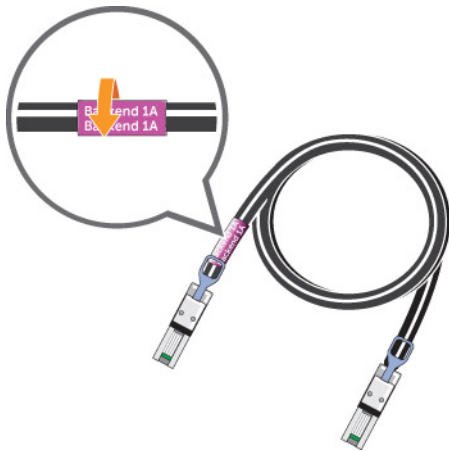
Figure 80. Wrap Label Around Cable
