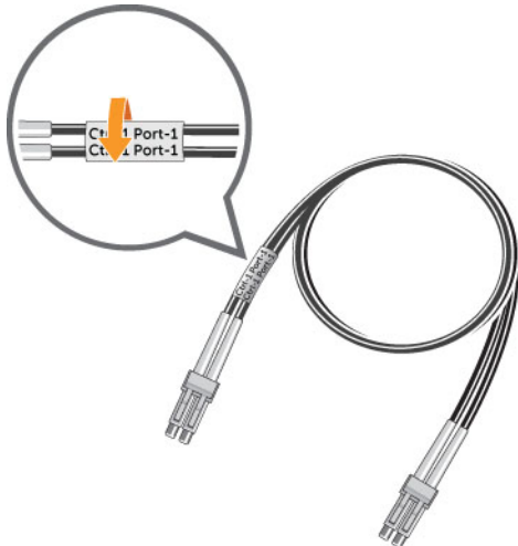
Figure 36. Wrap Label Around Cable
