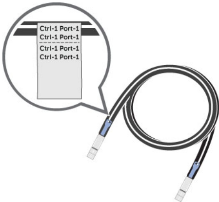
Figure 48. Attach Label to Cable
