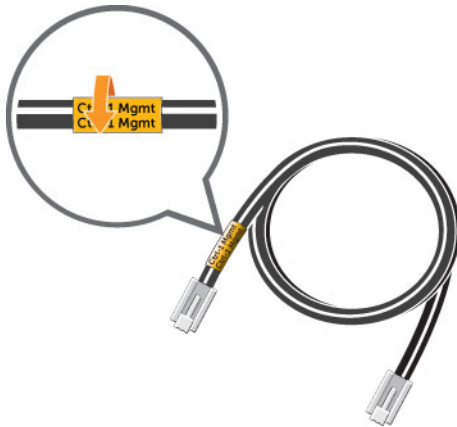
Figure 52. Wrap Label Around Cable
