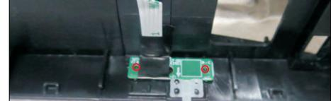
S13 Tear off tapes, then lift up the panel with the bracket for releasing the front bezel away from the panel.
