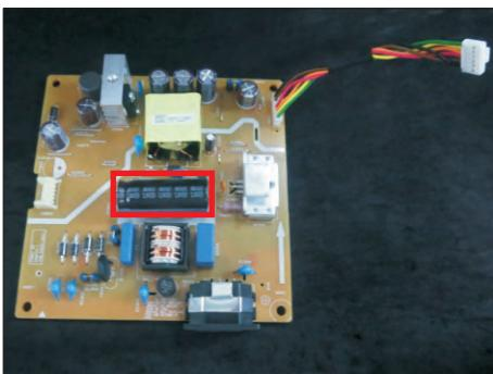
S20-4 Take out bulk cap. pin solder with soldering iron and absorber.
