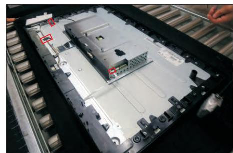
S12 Take away the middle bezel, and put it on a fixture, then tear off the mylar tape for releasing the LED board .
