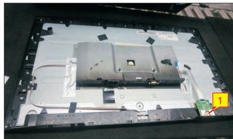
S9 Tear off 2pcs aluminium foils and 1pcs conductive tape for unfixing the bracket. Use a Philips-head screwdriver to remove 2pcs screws for locking the middle with the front bezel and the panel.
