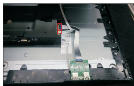
S7 Use a Philips-head screwdriver to remove 2pcs screws for unlocking the joystick key board unit, then tear off the tapes and release the USB board.
