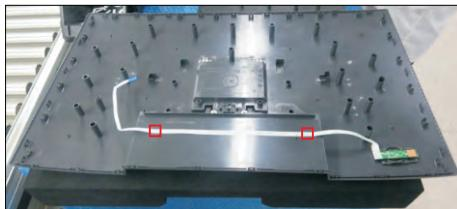
S8 Use a Philips-head screwdriver to remove one screw for unlocking the USB board unit, then release the USB board unit and put it aside.
