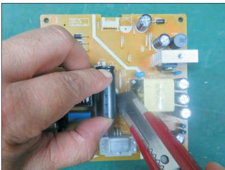
S20-5 Lift the bulk cap. up and away from the PCB.
