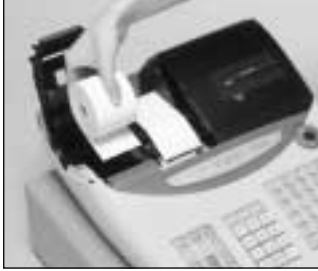
Step 3 Ensuring the paper is being fed from the bottom of the roll, lower the roll into the space behind the printer.
