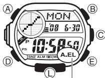
Auto light switch on indicator
