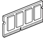
The printer has 32 MB (HL-3045CN) or 64 MB (HL-3075CW) of standard memory and one slot for optional memory expansion. You can expand the memory up to 544 MB (HL-3045CN) or 576 MB (HL-3075CW) by installing a Dual In-line Memory Module (SO-DIMM).
