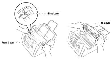
Pull the jammed paper gently from the paper feeder toward the back of the fax machine. If the paper remains jammed, then pull it toward the front of the machine.
