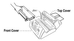
Remove the plastic stopper from the new print cartridge.
