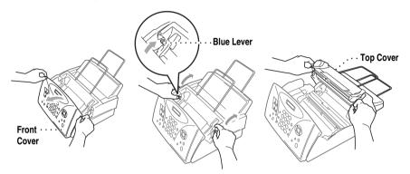
Remove the old print cartridge containing the used ribbon and dispose of it.
