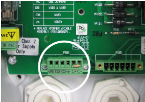
Figure 2.1 P106 connector with 100 Ohm resistor
