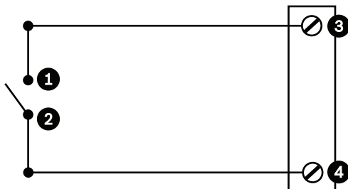
Figure 9.2 N.O. - Normally Open
