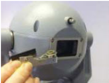
Figure 2.9: Remove wiper-arm from wiper shaft
