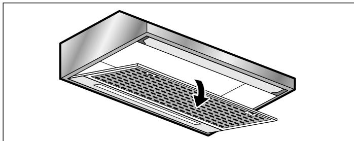
3. Position the filter grille at an angle and remove it.
