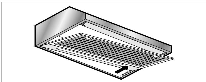
4. Remove the wires and then the metal filter mat.
