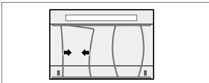
5. After removing the metal grease filter, clean the inside of the appliance.
